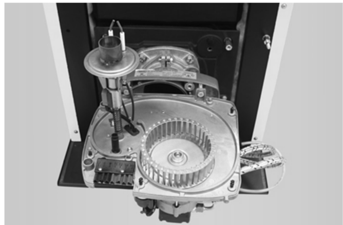
Abb. 27: Brenner in Serviceposition
